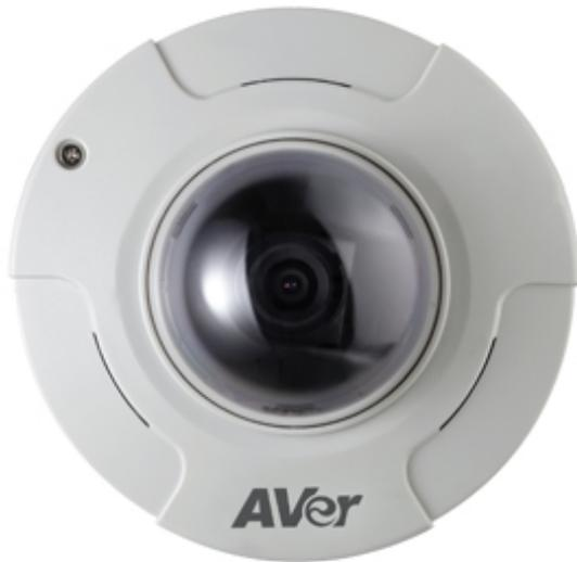
The full HD 2M FD2000 ceiling dome features a uniquely compact (97 mm diameter) and lightweight (380g) design for discreet surveillance in locations with strict space restrictions. The FD2000 is a perfect match for small boutiques, retail stores, restaurants and elevators, blending into a location's existing interior design to hide in plain sight. The pre-equipped recessed ceiling mount allows for easy and intuitive installation and is ideal for drop ceilings commonly seen in retail space.
